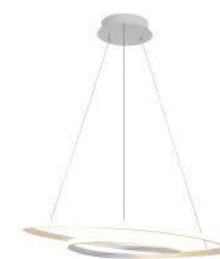
Sospensione / pendant lamp MD17011011-1A 3000K LED/54W, 3000K – lumen 4860, Dimmable ø cm 60 x H. cm 150, Class I, IP20
